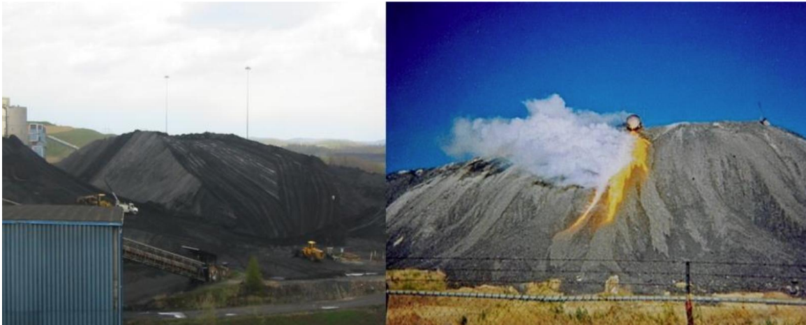
Figure 3 Dumping of induction furnace slag
