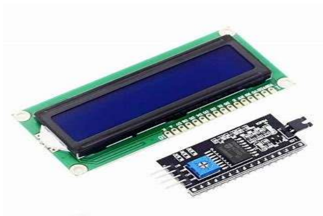
Fig 20. LCD Display with i2c pack
