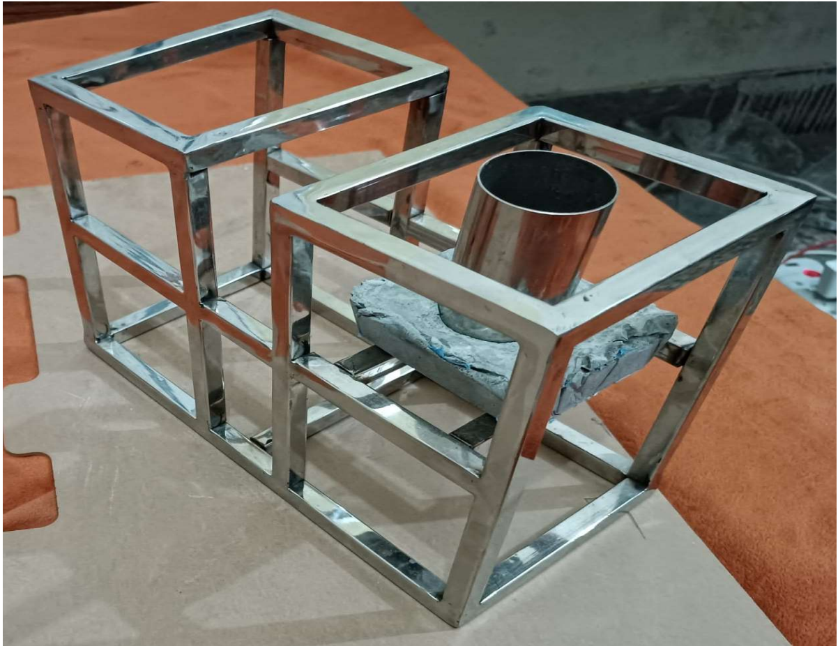
Fig 14. Steel cup, mortar insulation and chassis
