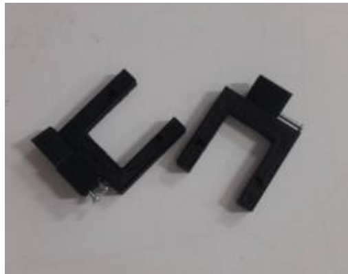
Figure 31 3D Printed and Connected TieRod and Connecting Rod
