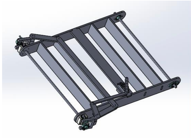
Figure 20 CAD model for Base of Mobile Platform
