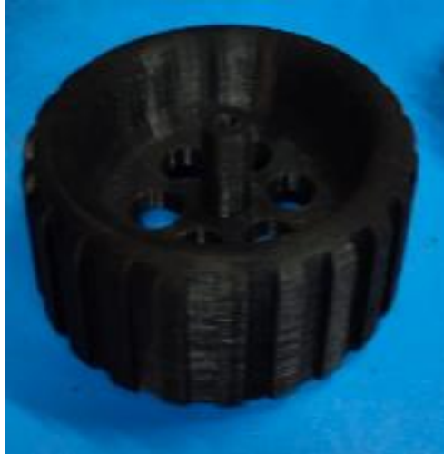
Figure 30 3D printed Wheel
