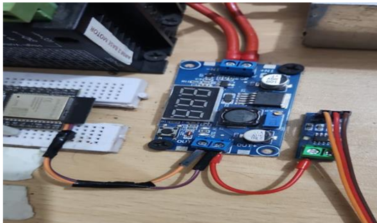
Figure 8: Buck Converter (Left), Current Sensor (Right)
