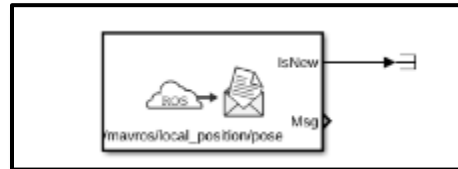
Figure 42 Subscriber block from ROS toolbox in Simulink
