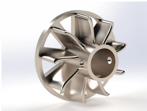
Figure 2 CAD Rendering of the final rotor design (front)
