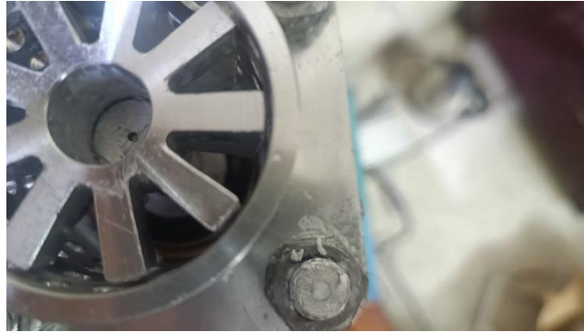
Figure 20 Close-up picture of rotor-stator shear gap
