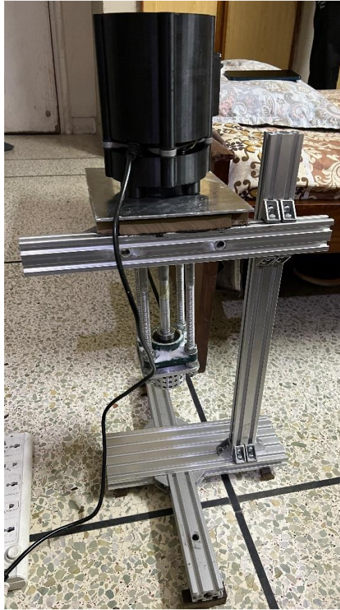
Figure 17 Final Homogenizer Assembly (View 1)
