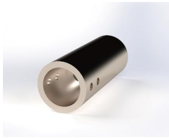
Figure 8 Motor-shaft coupling design (View 2)
