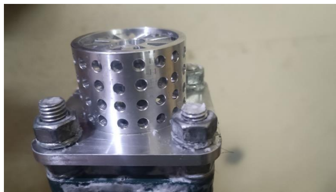
Figure 19 Close-up picture of stator
