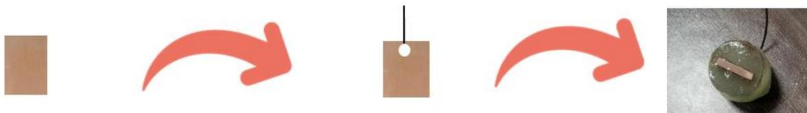
*Figure 4: Schematic illustration of cold mounting and hydrogel coating on copper electrode*
