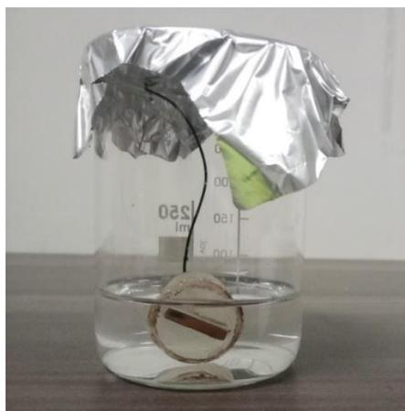
Figure 5: Hydrogel Coated Electrode dipped in Electrolyte (PBS)
