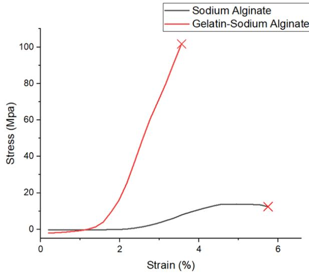
Figure 16: Tensile Test of Sodium Alginate and Gelatin-Sodium Alginate Hydrogel
