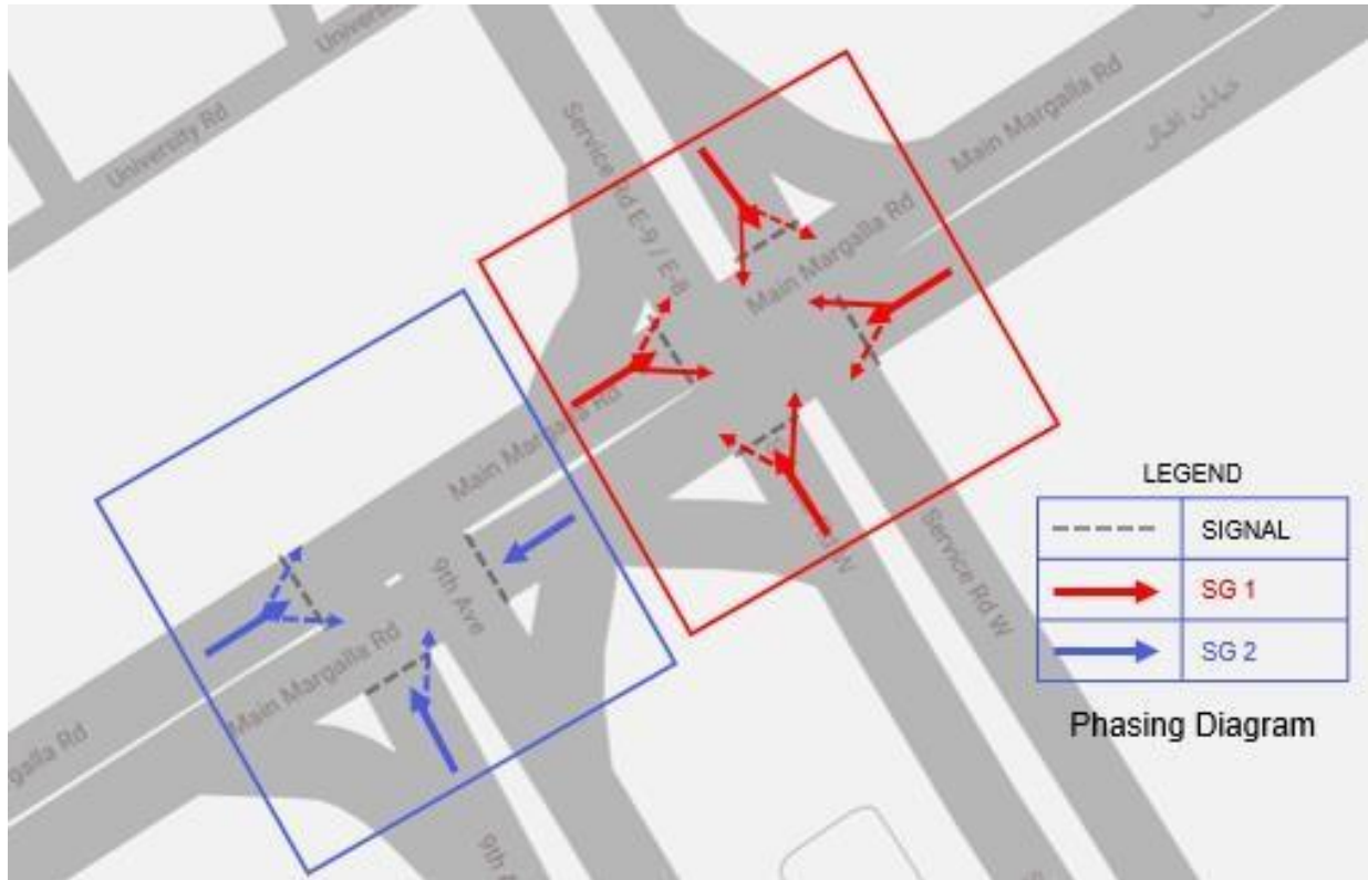
Figure 3-5: Split Phasing Design of 9 th Avenue Intersection
