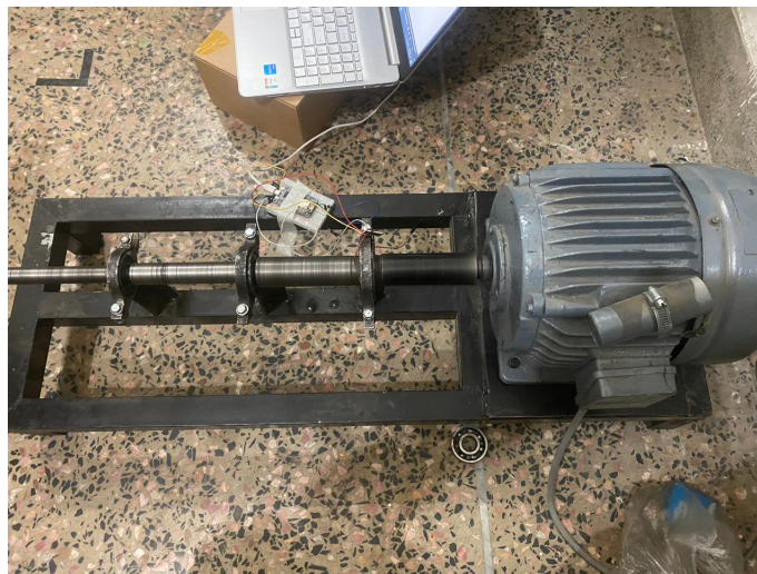
Figure 3.1: Test Rig with motor on it having extended shaft on which three bearings of different diameters are fixed through clamps
