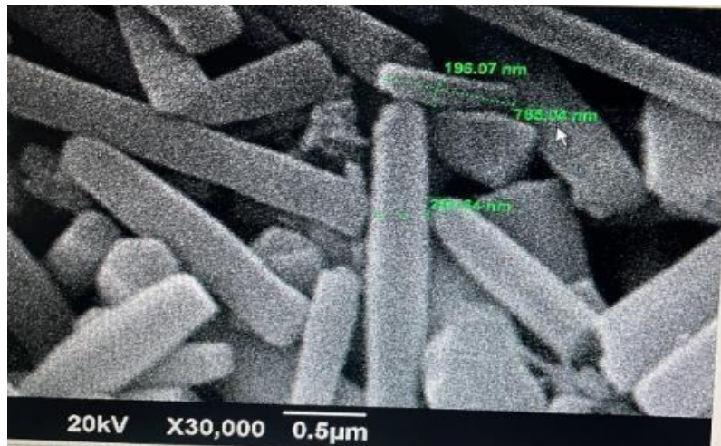
Figure 5 SEM image 2 of SiC whiskers
