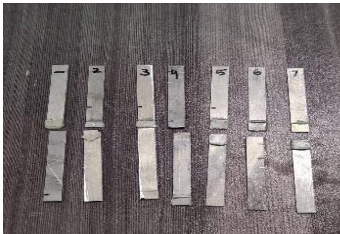
Figure 3 Sample preparation for adhesion test
