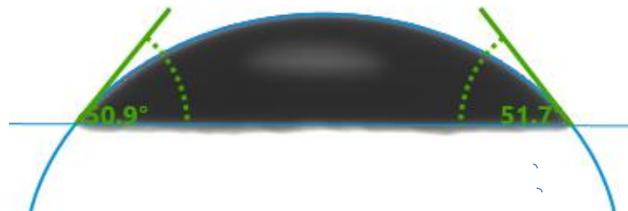
FIGURE 22 FIRST VALUE OF CONTACT ANGLE OF TREATED POLYMETHYL METHACRYLATE (PMMA) FOR 15 MINUTES, HAVING AN AVERAGE VALUE OF 51.3°
