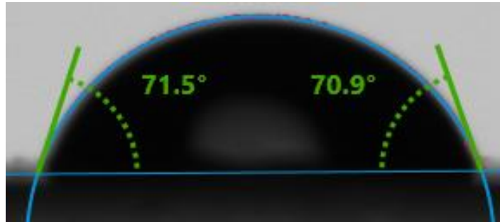
FIGURE 21 VALUE OF CONTACT ANGLE OF UNTREATED POLYMETHYL METHACRYLATE (PMMA), HAVING AN AVERAGE VALUE OF 71.2°
