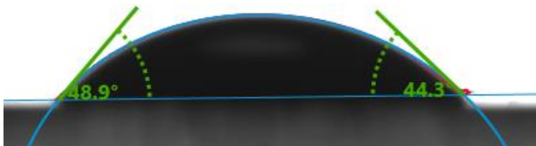
FIGURE 24 VALUE OF CONTACT ANGLE OF TREATED POLYMETHYL METHACRYLATE (PMMA) FOR 45 MINUTES, HAVING AN AVERAGE OF 46.6
