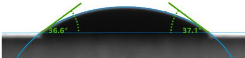
FIGURE 35 VALUE OF CONTACT ANGLE OF TREATED POLYMETHYL METHACRYLATE (PMMA) FOR 60 MINUTES WITH WATER, HAVING AN AVERAGE VALUE OF 36.85°
