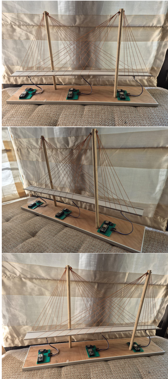
Figure 5.1: The Model Bridge with IoT network deployed
