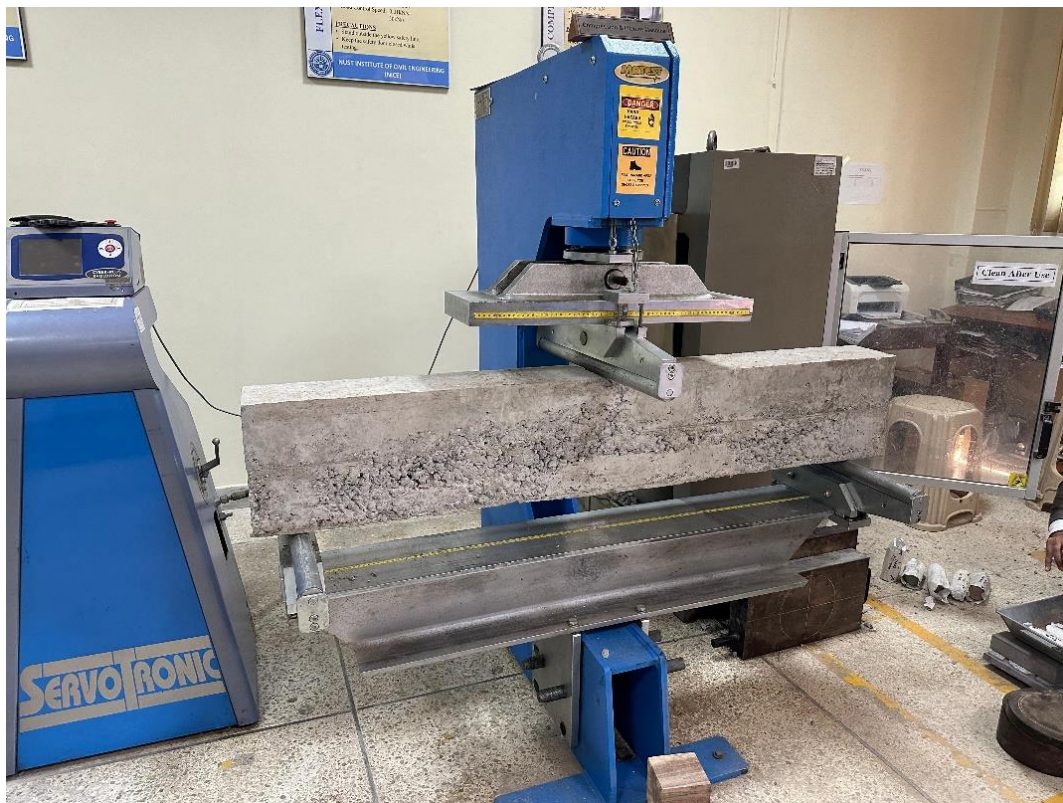
Figure 3: Midpoint Testing of Beam
