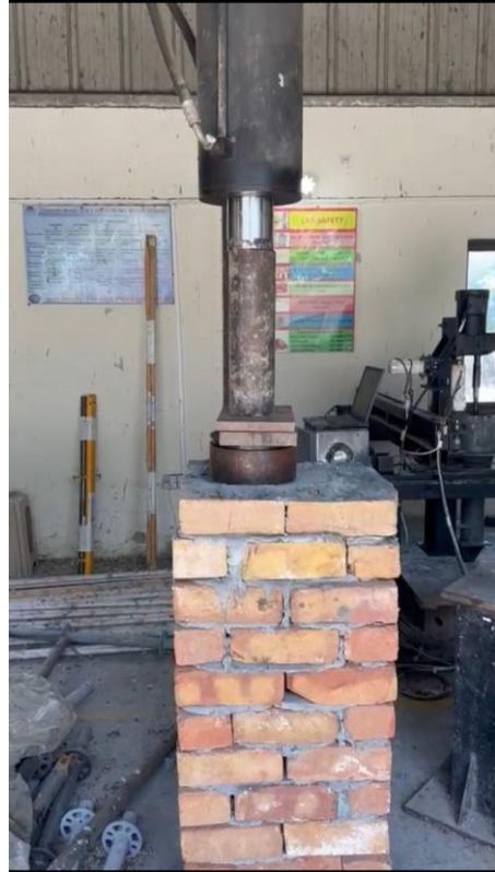
Figure 6: Testing of Column
