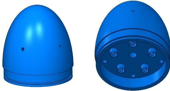
Figure 5.2: 3D Printed AUV Nose with holes for ballast system
