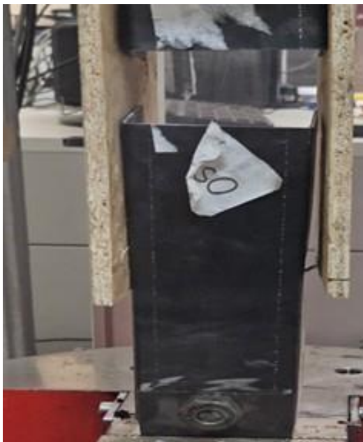
(a) OSB-1 pull-through failure (PT)
