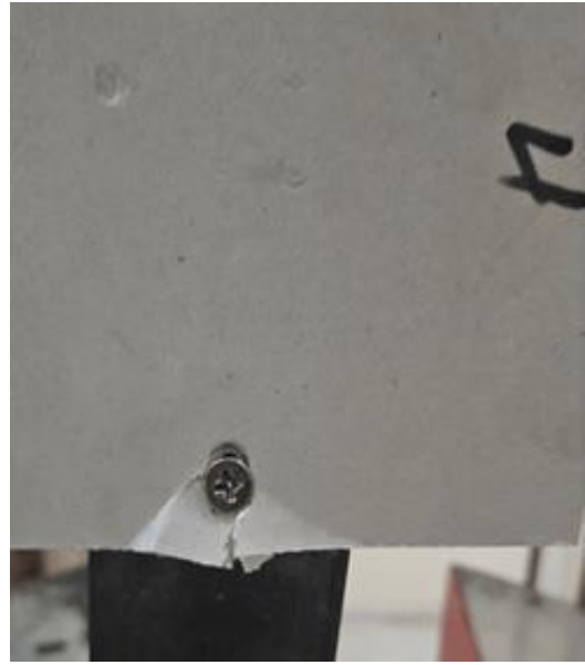
(l) GYP-4 bearing failure/ edge-tearing (B+E)
