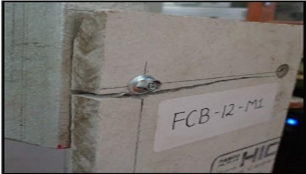
Figure 1.12: Tensile crack under screw location
