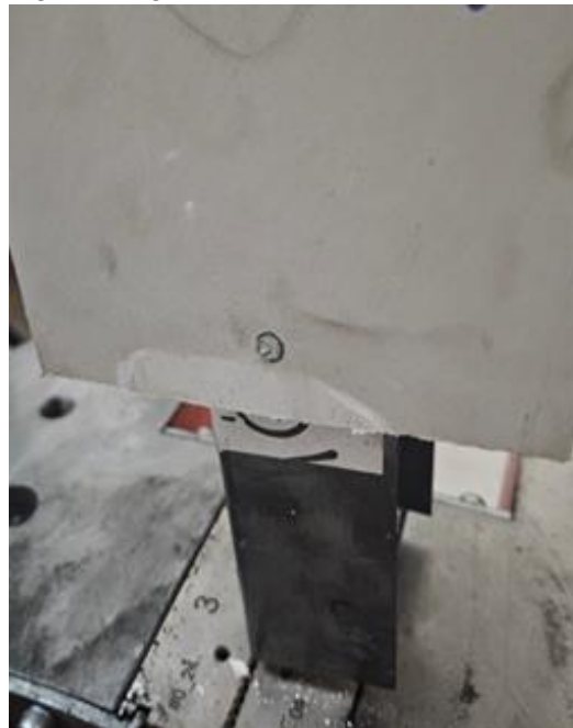
(m) GYP-5 bearing failure/ edge-tearing (B+E)
