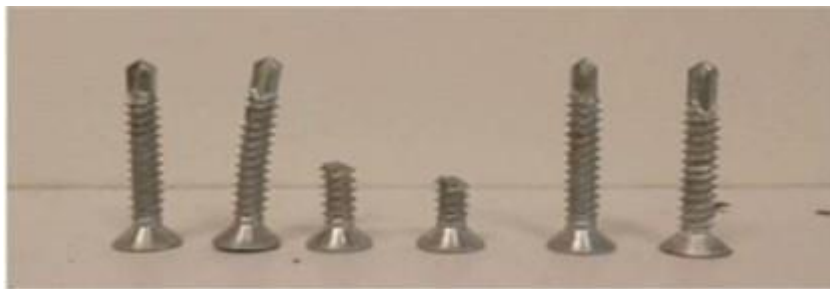
Figure 1.11: Bending and shearing off
