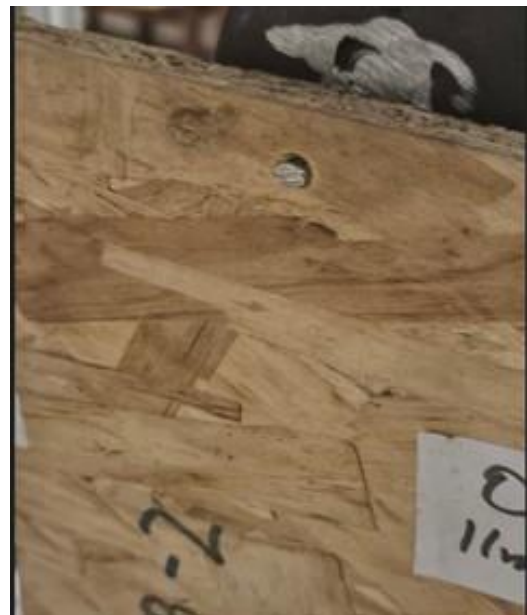
(b) OSB-2 bearing failure (B)
