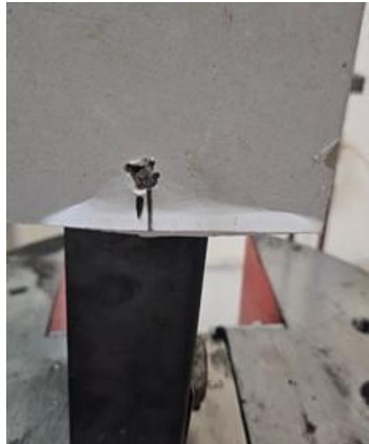
(j) GYP-2 bearing failure/ edge-tearing (B+E)
