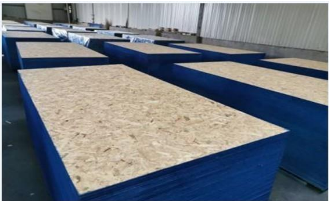
Figure 1.5: 11mm/12mm/15mm/18mm OSB Manufacturer Oriented Strand Board Sandwich Panel [1]
