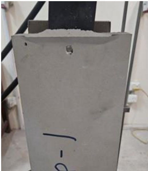
(i) GYP-1 bearing failure/ edge-tearing (B+E)
