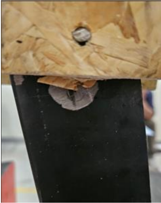
(c) OSB-3 back-edge tearing combined with tearing(PT+E)
