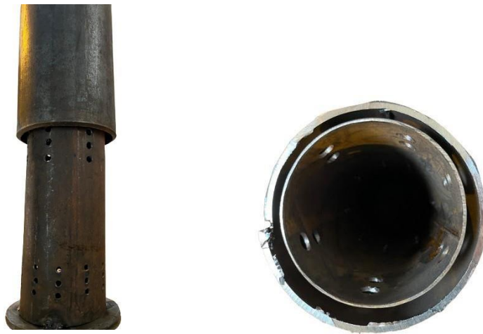
Figure 14(a & b): Combustion Chamber
