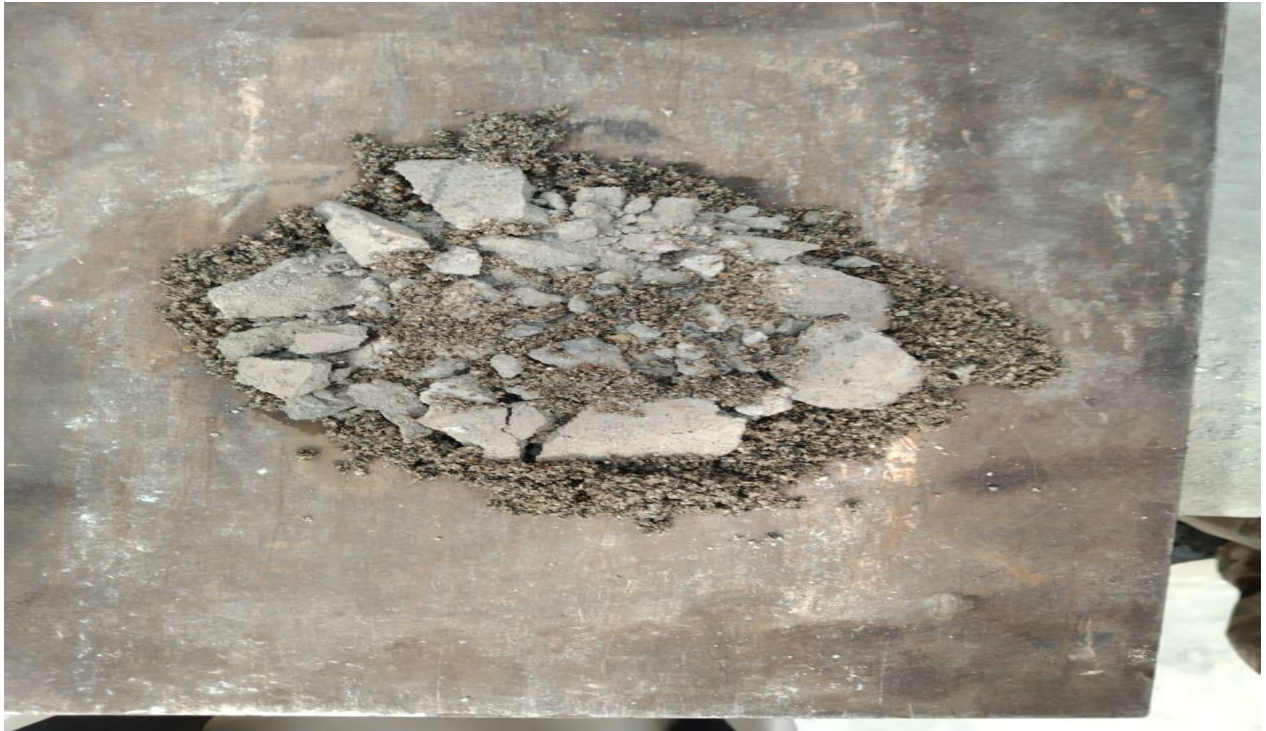
Figure 4.2 Compressive Strength Test Sample
