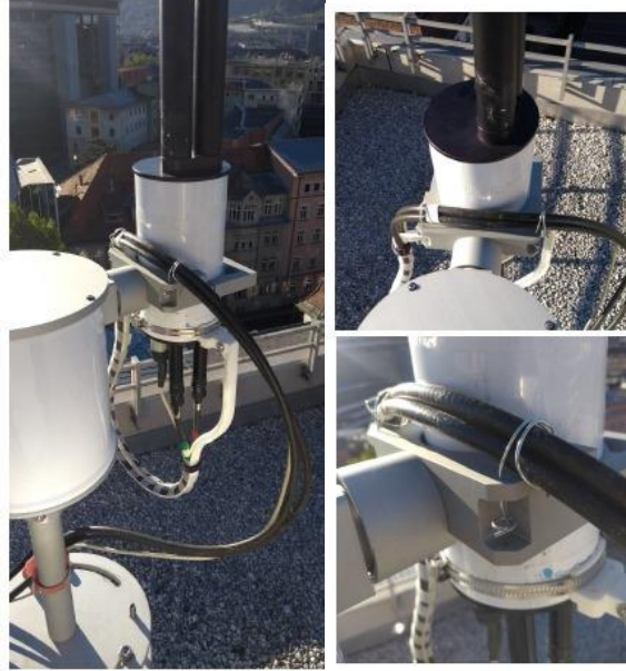
Figure 14: NASA Pandora Spectrometer Fiber Cable Layout
