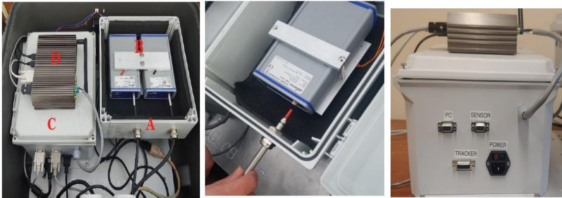
Figure 13: NASA Pandora Main Control Unit Components
