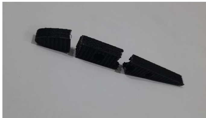
Figure 32 3-Point Bend Testing Performed on Weakest Rib
