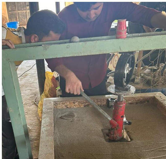
Fig 7 showing load being applied on foundation resting on sand through hydraulic jack.
