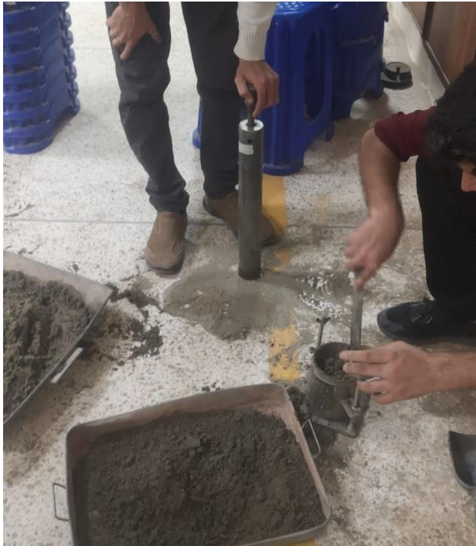
Fig 4 Showing preparation of test mold and test samples for Performing Proctor test.
