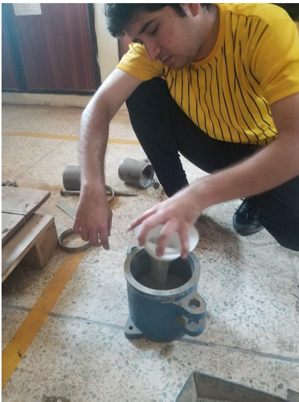
Fig 5 Showing preparation of test mold and test samples for Performing Relative density test.
