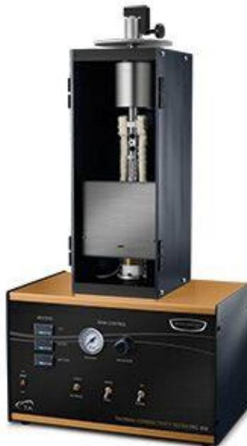
**Figure 2. 14:** Guarded heat flow meter[57]
