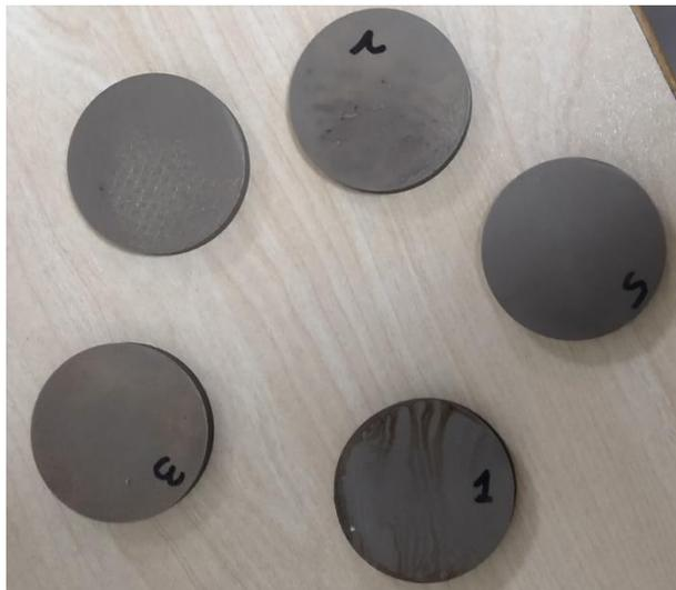
**Figure 2. 13:** samples for thermal conductivity test
