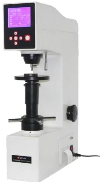
**Figure 2. 12:** Rockwell hardness tester machine[56]
