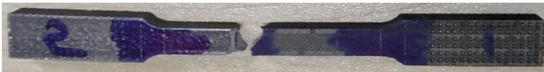
Figure 3. 4: Fracture of tensile testing sample at room temperature
