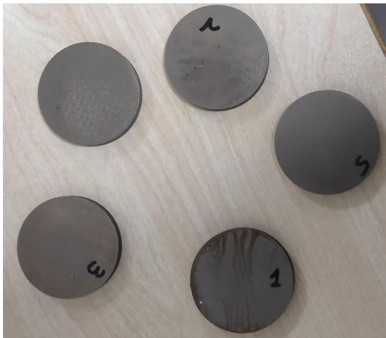
**Figure 3. 2:** 3D Printed sample by FARSOON Machine
