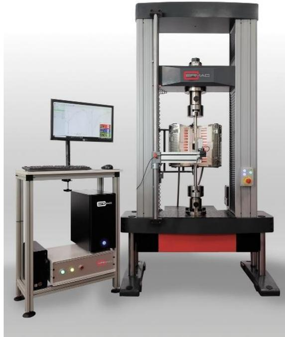
**Figure 2. 8:** UTM with furnace for elevated temperature testing[51]
