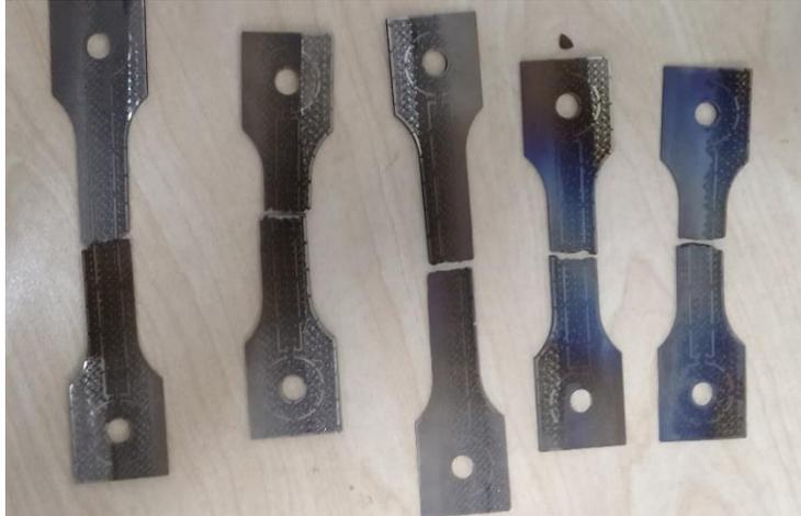
**Figure 2. 7:** samples for testing at elevated temperatures
