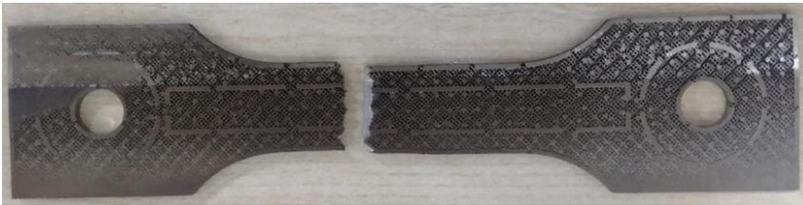
**Figure 3. 5:** Fracture of tensile testing sample at elevated temperatures
