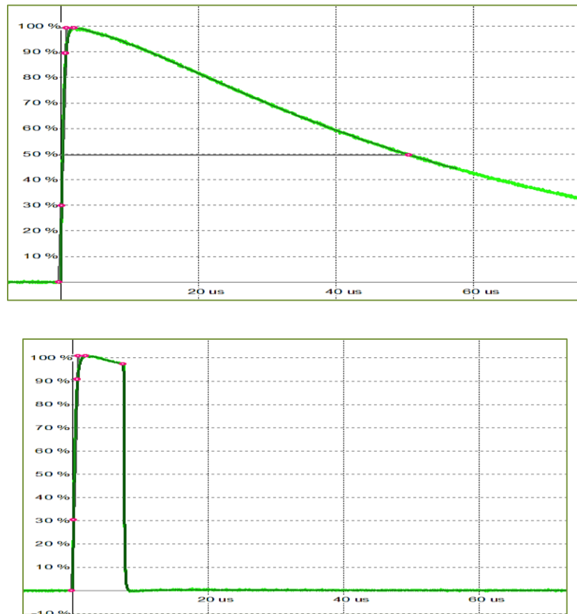
Figure 4.3: (a) Positive Lighting Impulse without breakdown (b) Positive lighting impulse with breakdown.
