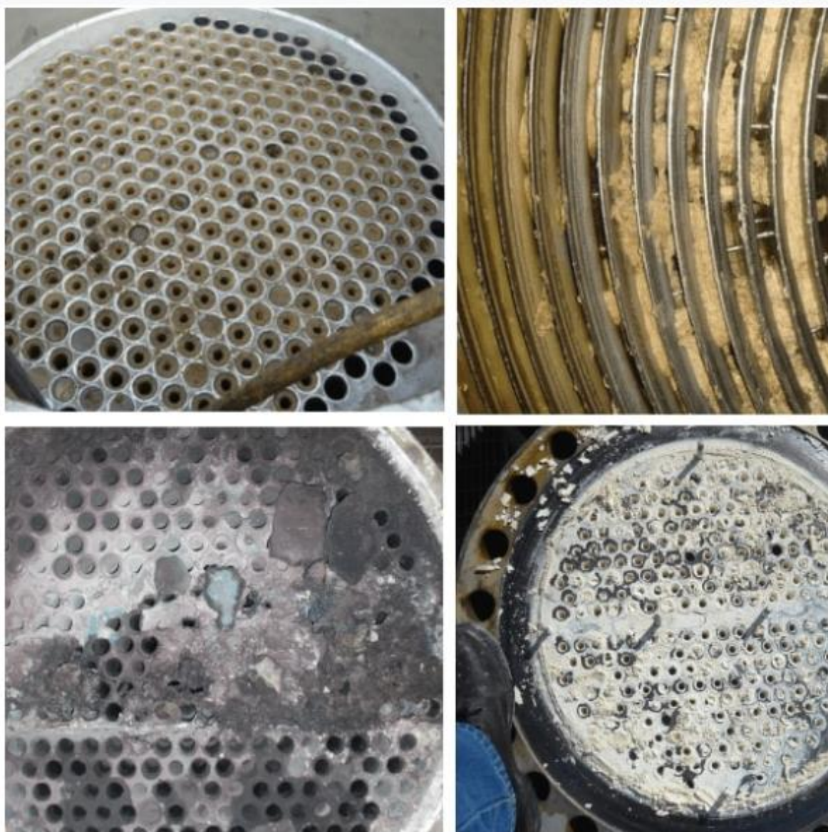
Figure 6: Fouling inside tubes of heat exchangers. *
