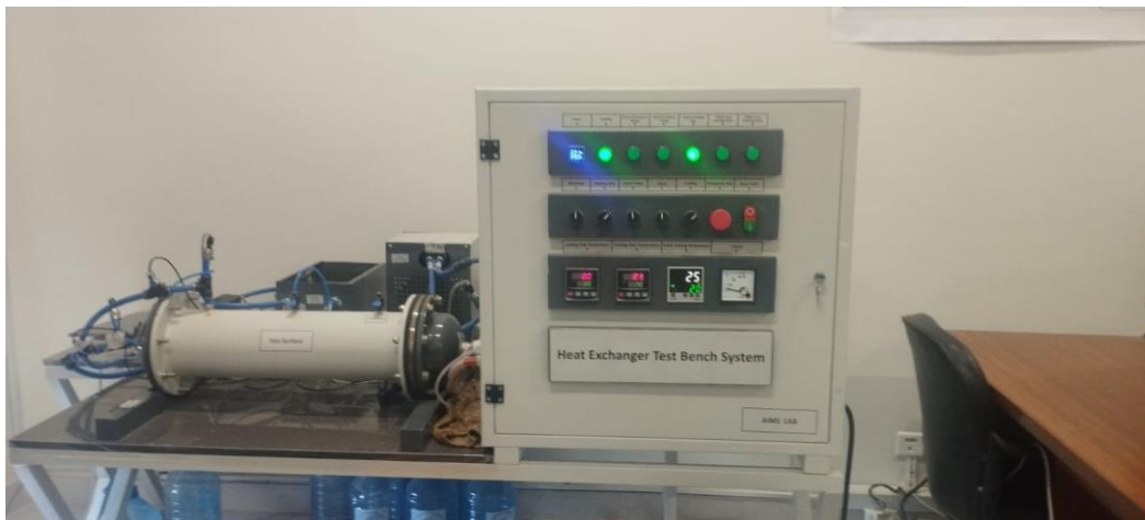
Figure 31: Cold Water at 27°C, Hot water at 70°C.
