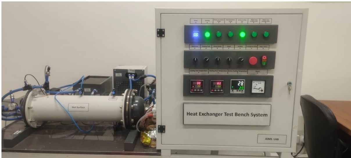
Figure 27: Cold water at 29°C, Hot water at 60°C.
