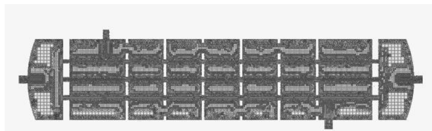
Figure 17: Overall Mesh of the heat exchanger.
