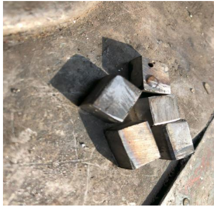
Figure 3.8: 5mm×11mm of steel samples
