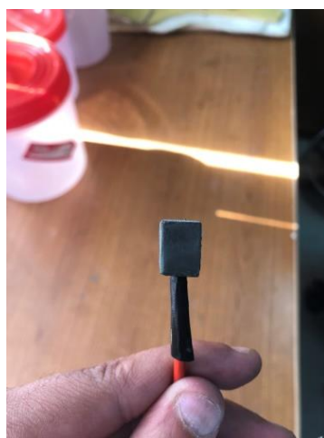
Figure 3.13: Coating deposited at peak current density
