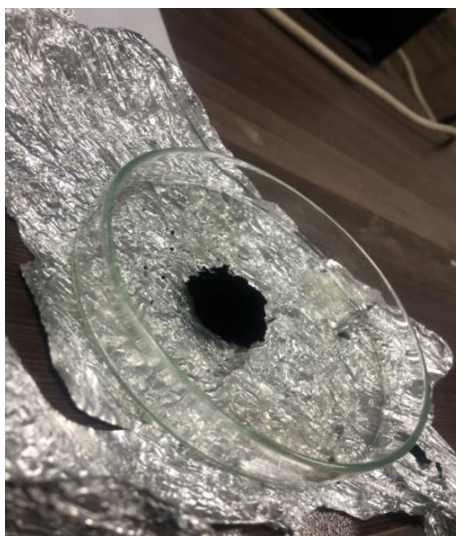
Figure 3.6: rGO in powder form
