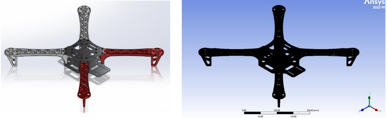
Figure 18: Drone Chassis and its Mesh
