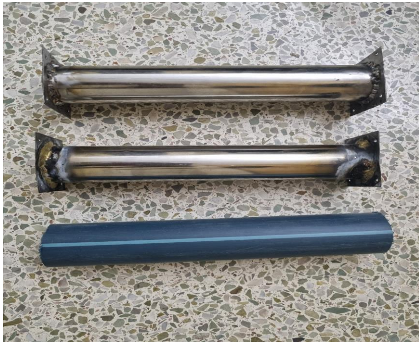
Figure 13: Stainless steel cylinder (top two) and PVC cylinder (bottom)
