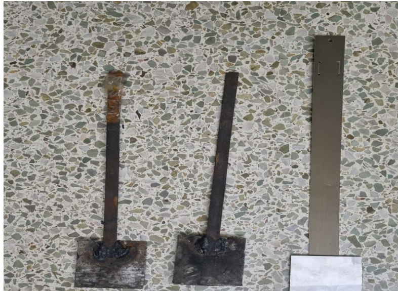
Figure 10: Aluminum sheet supports
