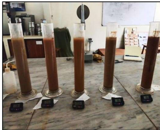
Figure 8: Hydrometer Analysis of Soil
