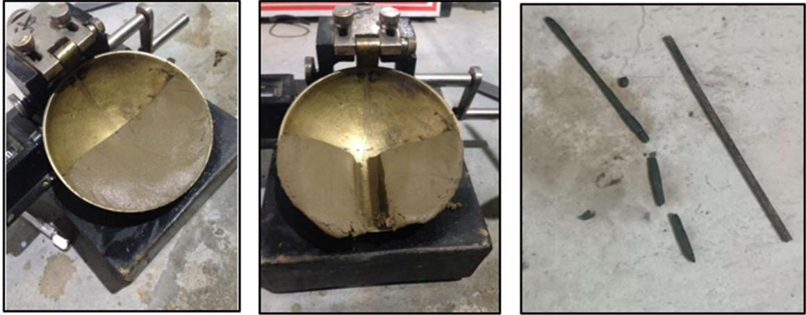
Figure 10: Atterberg limit test using casagrande method
