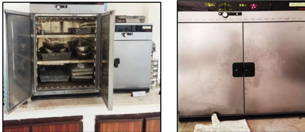
Figure 6: Oven used to find Natural Water Content of Soil
