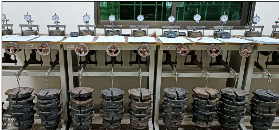
Figure 11: Oedometer test for C_c and C_v
