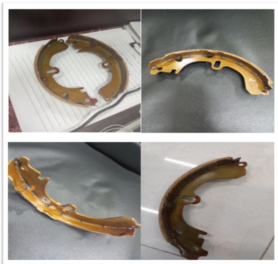
Figure 4.1. Images of counterfeit and original brake shoe from dataset collected
