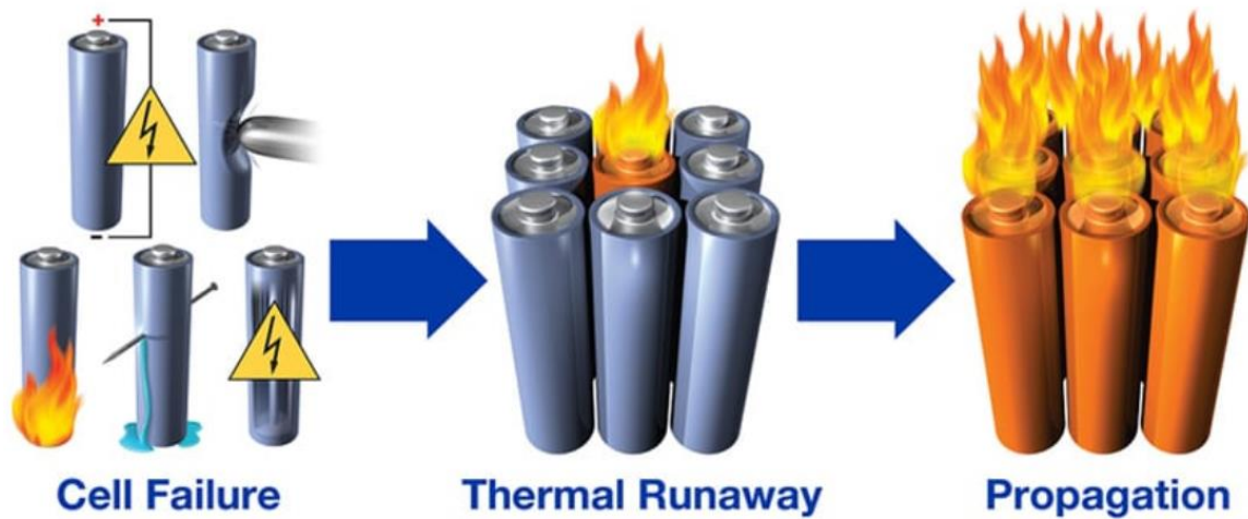
Figure 1.1.4: Failure to thermally manage the Lithium ion battery is show, ones the one cell thermally fails than the whole battery pack will fail and it will as a whole catch fire[3].
