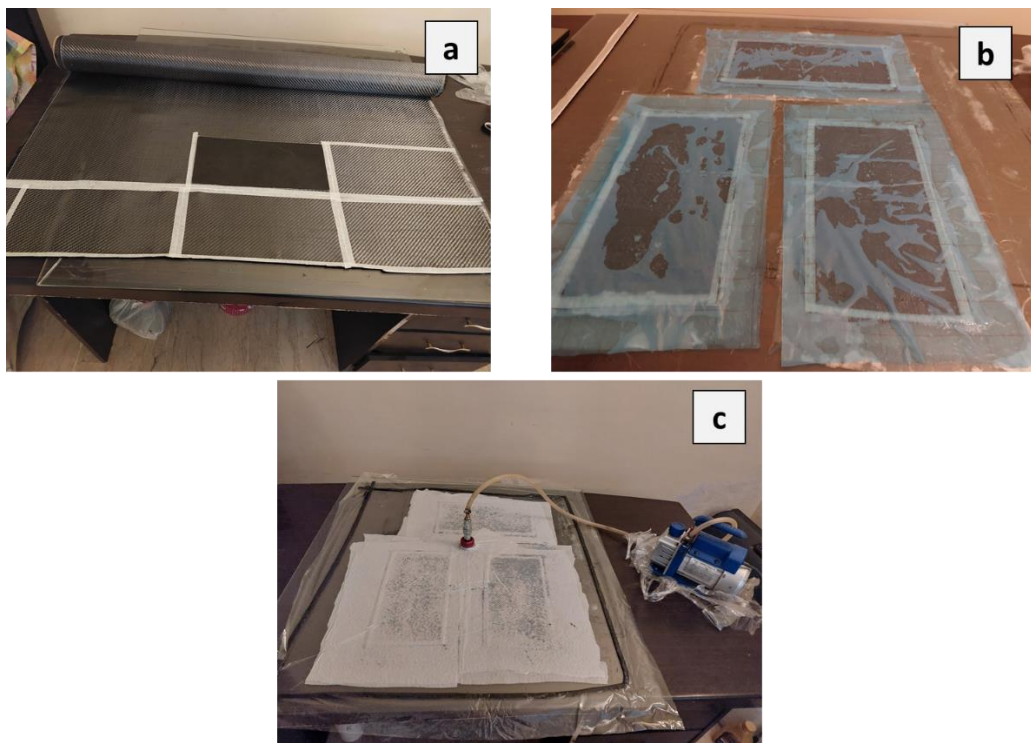
Figure 3.2: Vacuum Bagging Process for Manufacturing Sandwich Panel: a) Cutting Carbon Fabric into Small Pieces, b) Applying Epoxy & Adding Layers, c) Vacuum Creation to Remove Excess Epoxy
