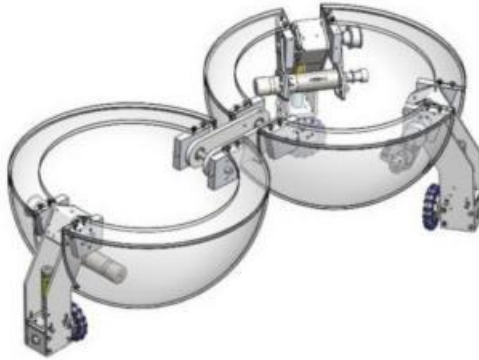
Figure 11 Image of spherical robot after reconfiguration
