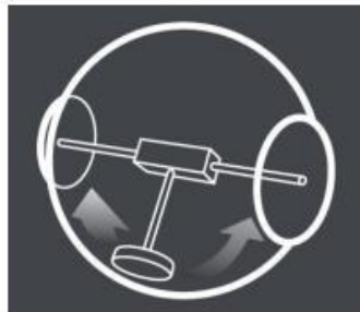
Figure 6 A commercialized pendulum-driven robot, Rotundus
