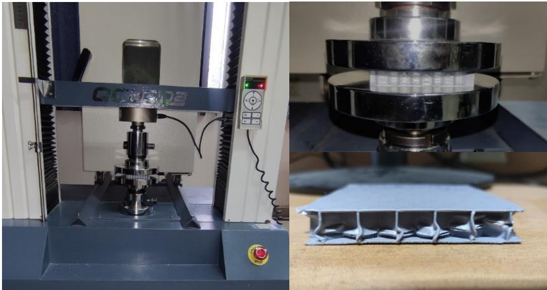
Figure 3-8 : Flatwise Compression Test
