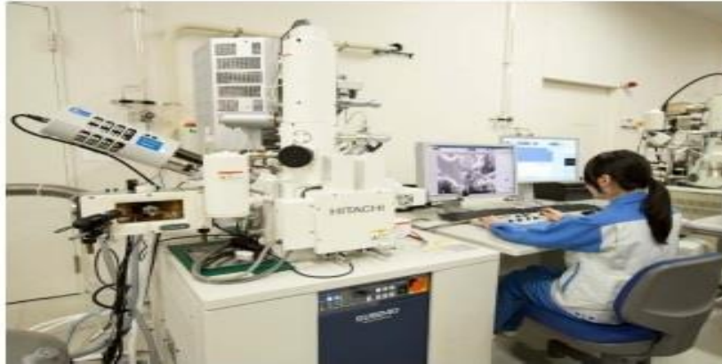
Figure 3.15: EDX measurement inside the SEM [100]
