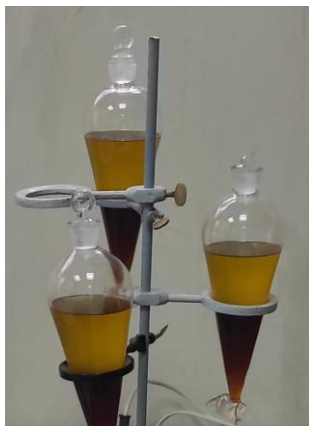
Figure 3.4: Formation of two layers impure biodiesel and glycerol [55]
