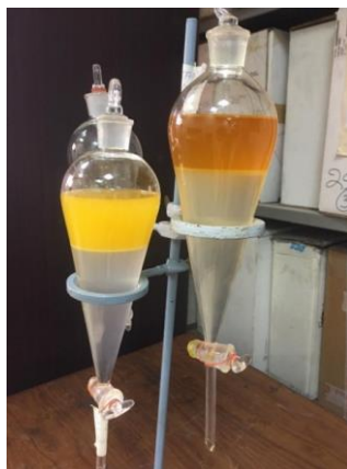
Figure 3.5: Biodiesel and water layers after three washes [55]
