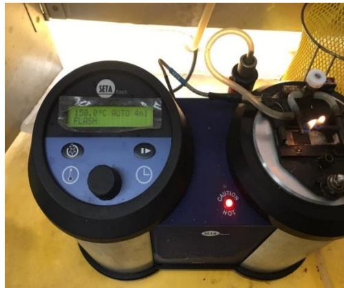
Figure 4.3: Flash Point Tester [55]
