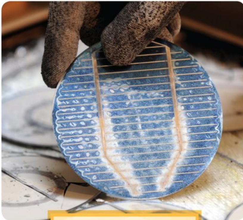
Silicon is removed from old solar panels and reused in new panels.
