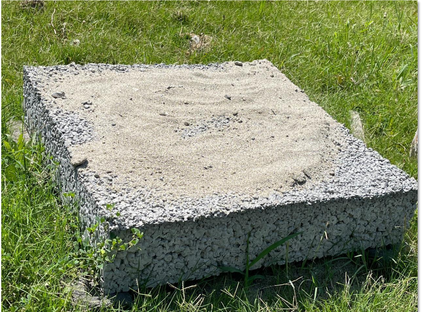
Figure 14: PCP exposed to dust and environment to check for clogging
