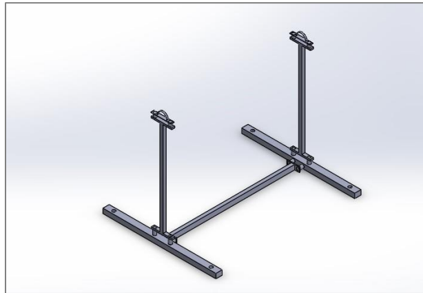
Figure 3.5: SOLIDWORKS Model of Support Structure for PTC
