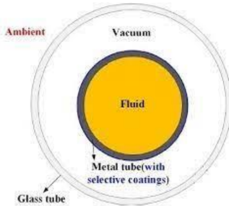
Figure 1.10: Evacuated Receiver Tubes [14]
