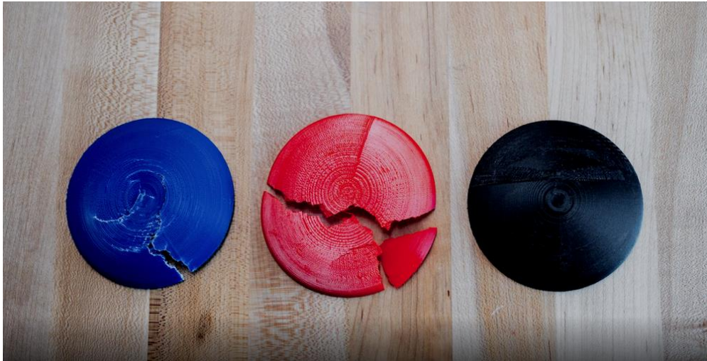
Figure 1: ABS (blue), PLA (red), and Kevlar-reinforced Onyx (black) parts struck with a hammer
