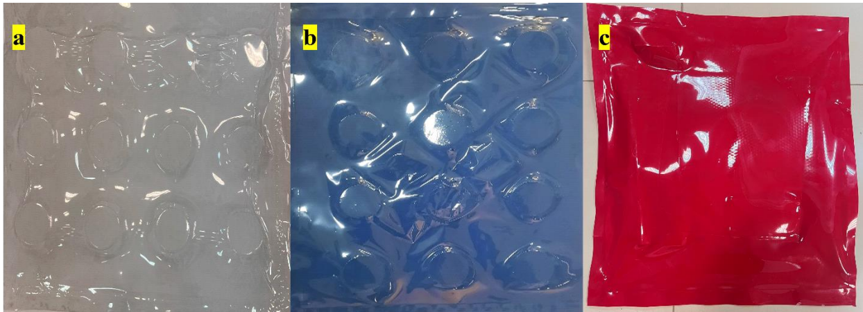
Figure 4.8: Plastic sheets unable to conform to the Mold shape due to insufficient heat.
