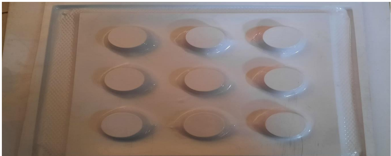
Figure 4.10: Wrinkles on Milky ABS sheet when distance b/w ups is 42mm
