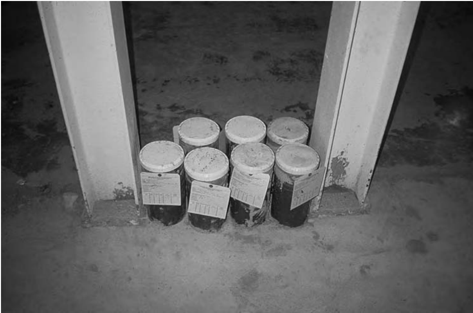
Figure 8.1 Concrete cylinders are used to determine compressive strength in many parts of the world. The UK uses cubes instead
