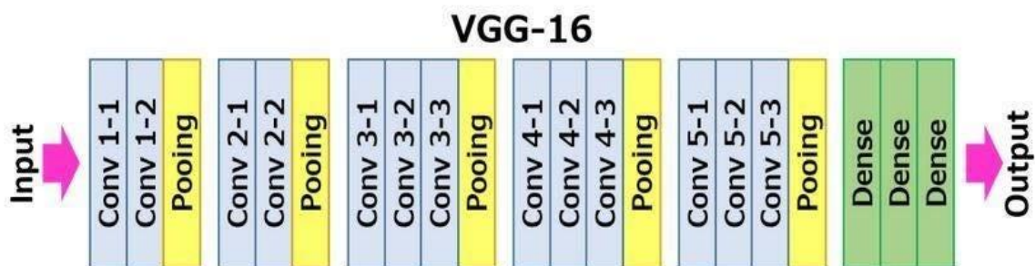
Figure 13: The VGG16 model for classification [21]
