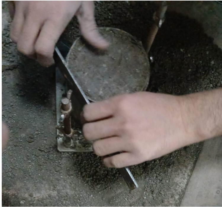
Figure 9: Proctor Test Apparatus
