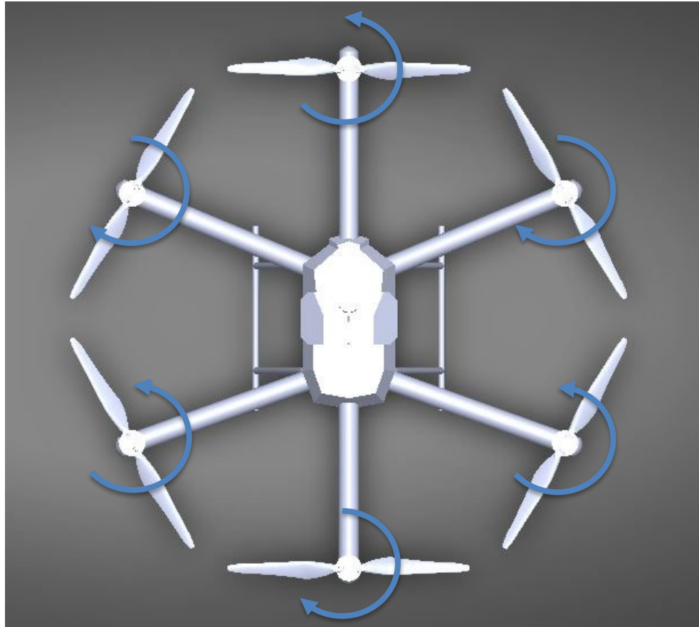
Figure 3.10 Rotational direction of each rotor in the Hexacopter
