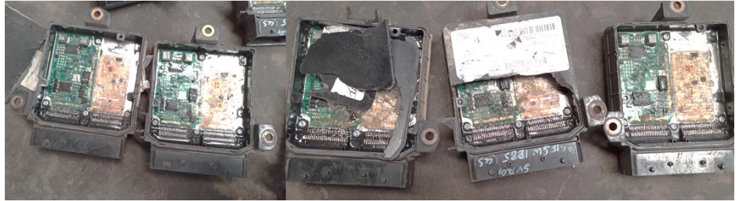
Figure 7 – Pictures of Faulty TCMs
