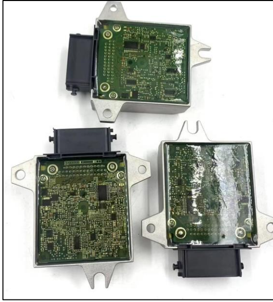
Figure 2 – Degraded TCM Circuits
