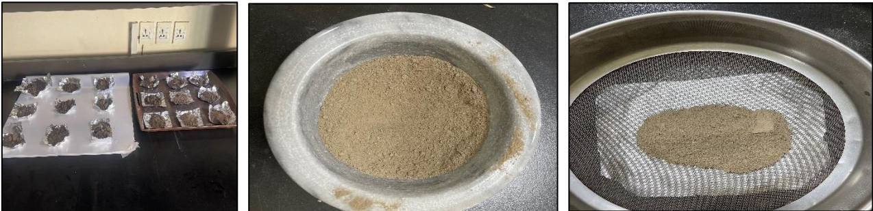
Figure 3.5: (A) Drying of soil samples (B) Grinding of soil samples (C) Sieving of soil samples for the digestion process
