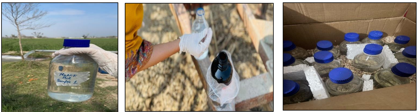
Figure 3.2: (A) Ground water collection (B) Water preservation with nitric acid (C) Stored water
