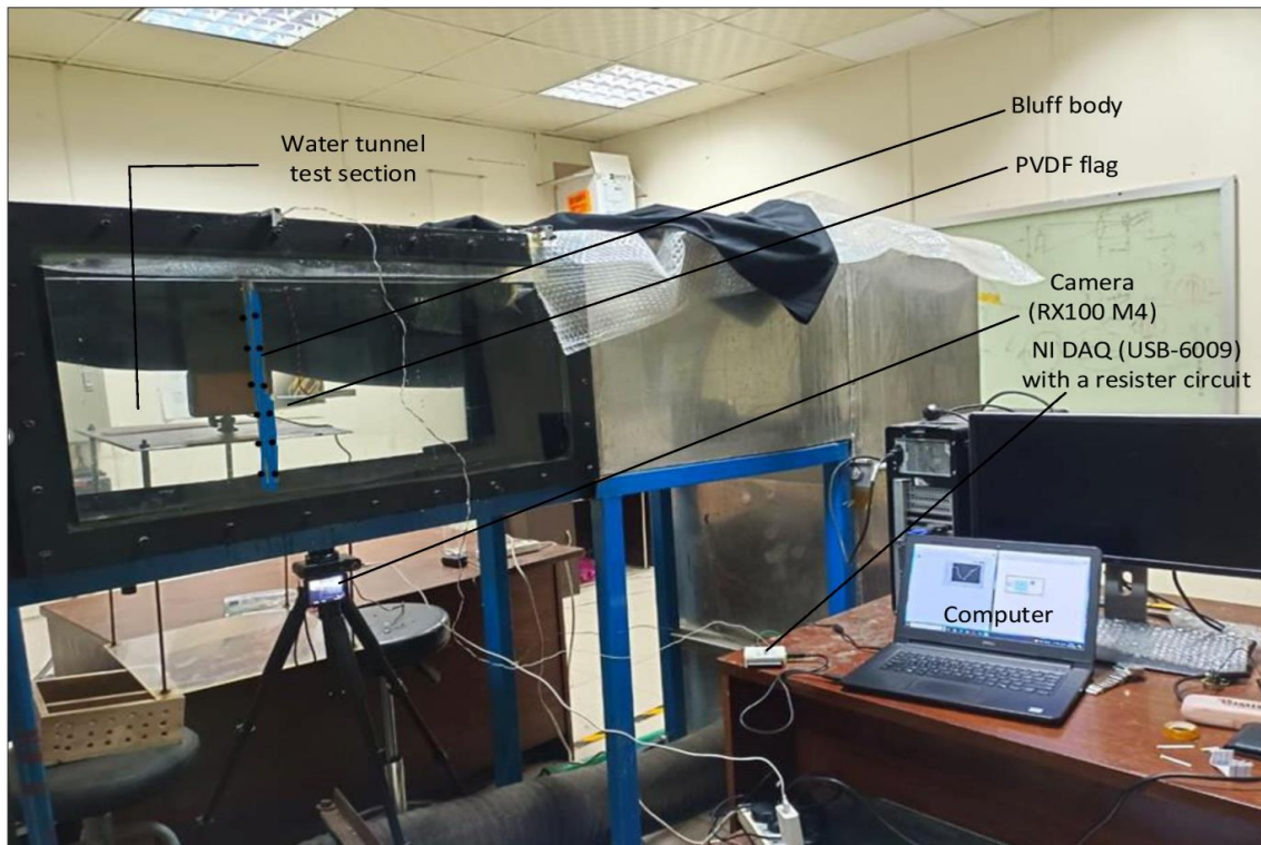
Figure 3.1: Experimental setup of flow lab.
