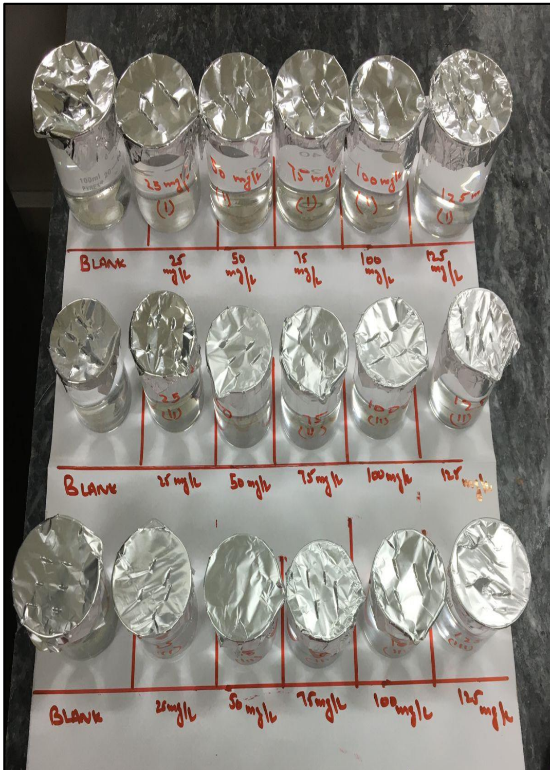
Figure 3.12: Exposure setup in triplicates for mono and coexposure of microplastics
