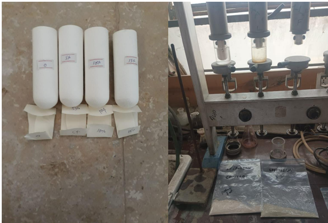
Fig 6: Crude Fat Test. The samples obtained using a Soxhlet equipment
