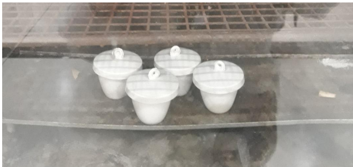
Fig 3: Spirulina samples being dried to remove moisture in hot air oven
