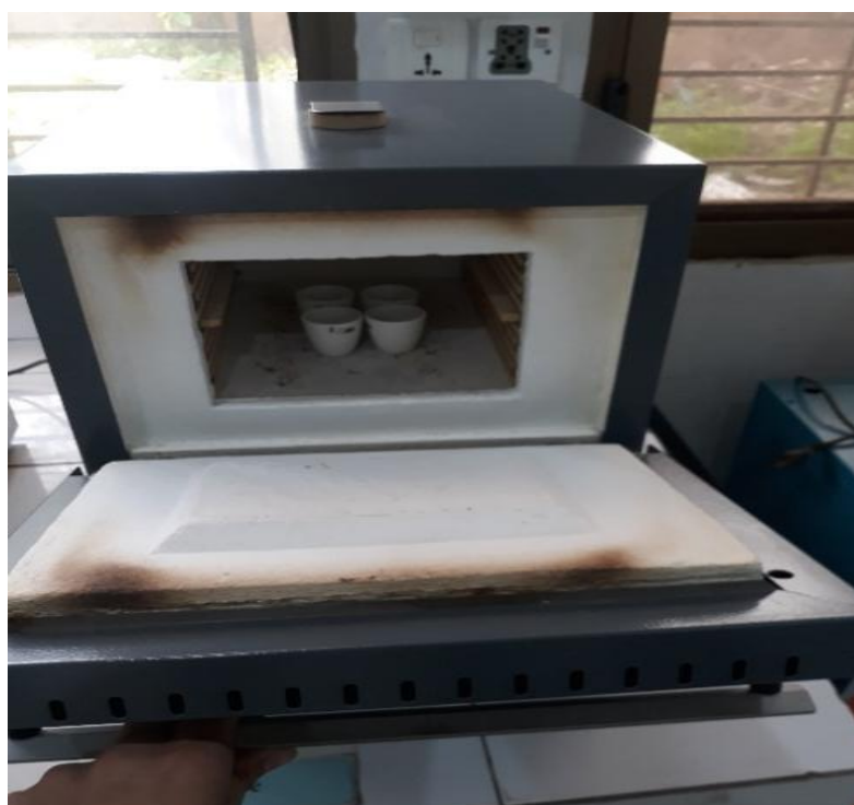
Fig 4: Displays the charred residue of the samples after undergoing treatment in the muffle furnace
