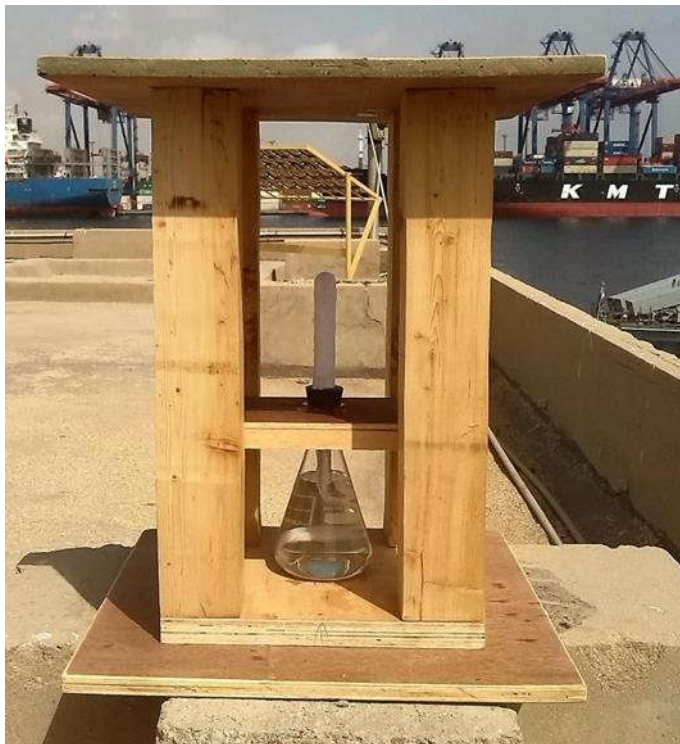
Figure 3-3: Wooden Frame Housing Conical Flask and Wet Candle for Determination of Atmospheric Chloride
