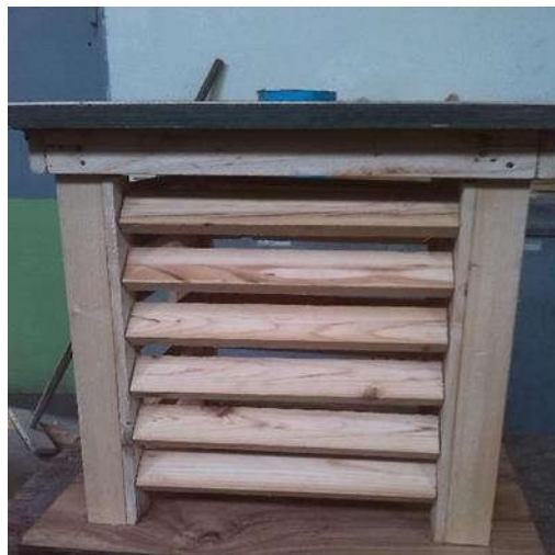
Figure 3-4: Wooden Frame Housing Sulfation Cylinder for Measuring SO 2 Concentration
