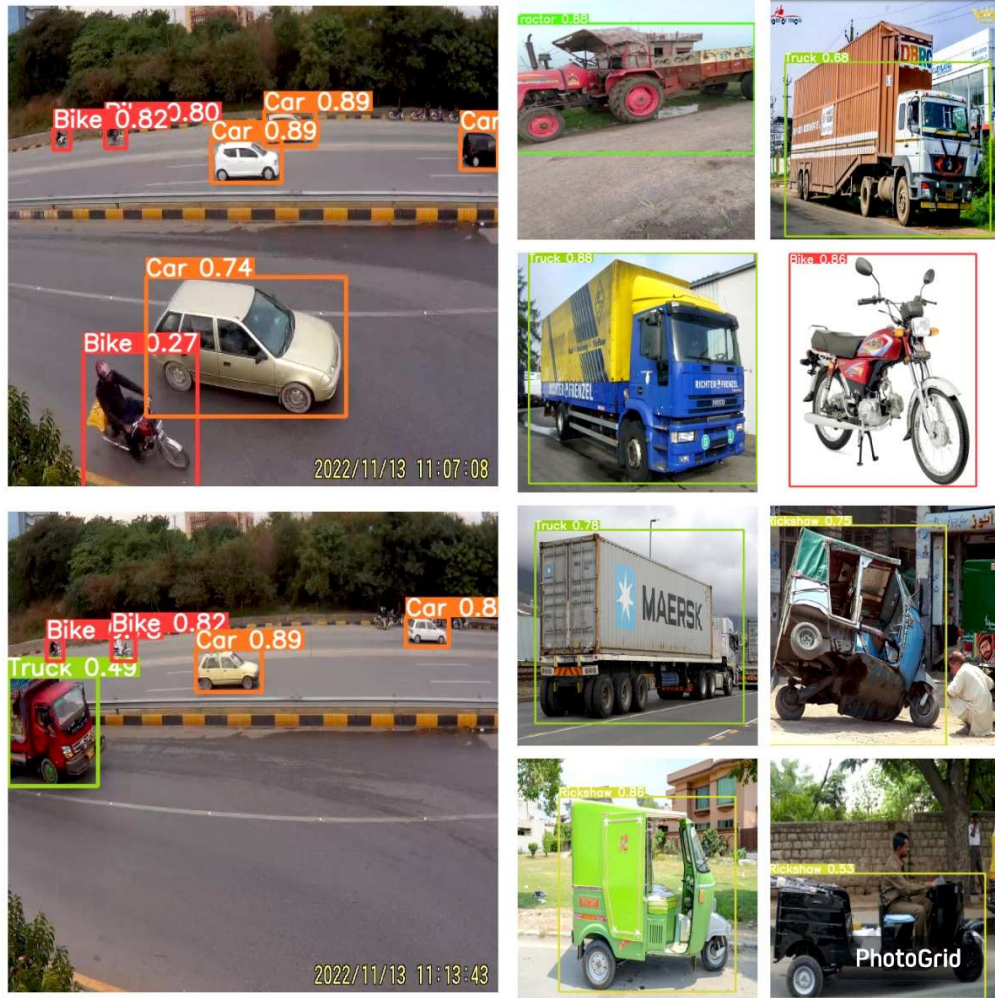
Figure 22: Inferences on test Images showing accurate detection of Bikes, Trucks, Rickshaws, Cars and tractors
