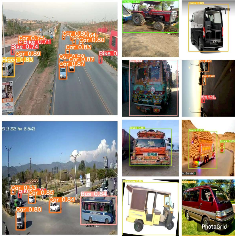
Figure 23: Inferences of test Images showing accurate detection of Bike, Cars, Trucks, Hiace, Rickshaws, Tractors and Buses
