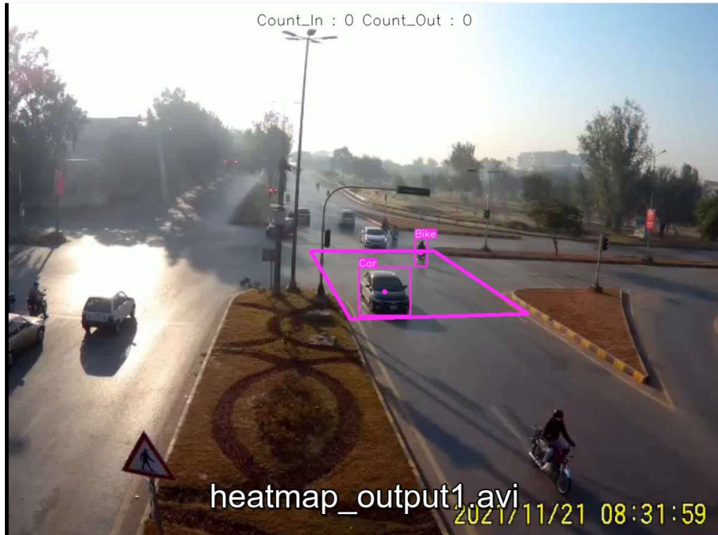
Figure 14: Image from an output video showing area of interest for traffic density estimation
